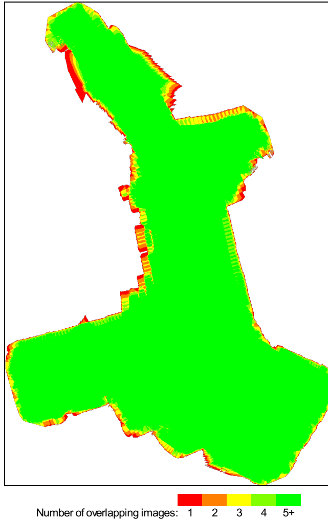
Figure 4: Number of overlapping images computed for each pixel of the orthomosaic. Red and yellow areas indicate low overlap for which poor results may be generated. Green areas indicate an overlap of over 5 images for every pixel. Good quality results will be generated as long as the number of keypoint matches is also sufficient for these areas (see Figure 5 for keypoint matches).
